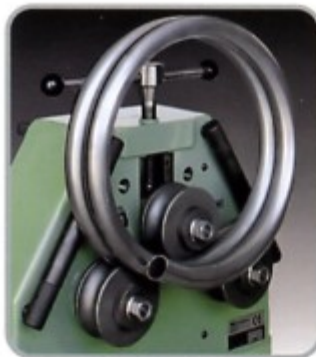
Rolling with Optional Tube Rolls Knurled / Smooth Available
