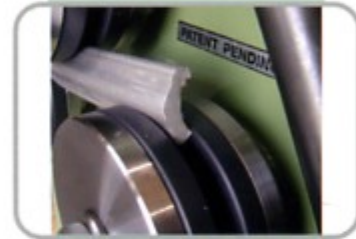
Special Rolls for Cap Rail Available in Steel & Polymer for Brass & Aluminum
