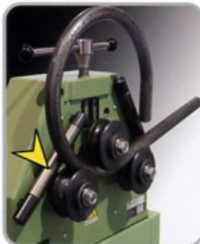
Standard Guides have Adjustable Rake Angle
