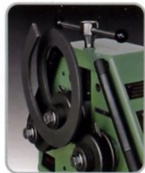
Rolling Bar On Edge (Hard Way), with Standard Rolls
