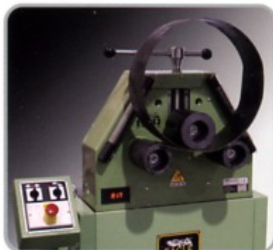
Rolling Wide Thin Sheet Material with Optional Wide Flat Rolls
