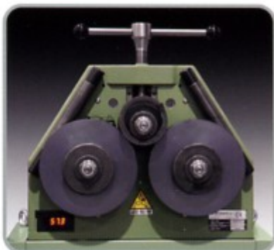
Rolling Small Rings with Optional Tight Diameter Rolls
